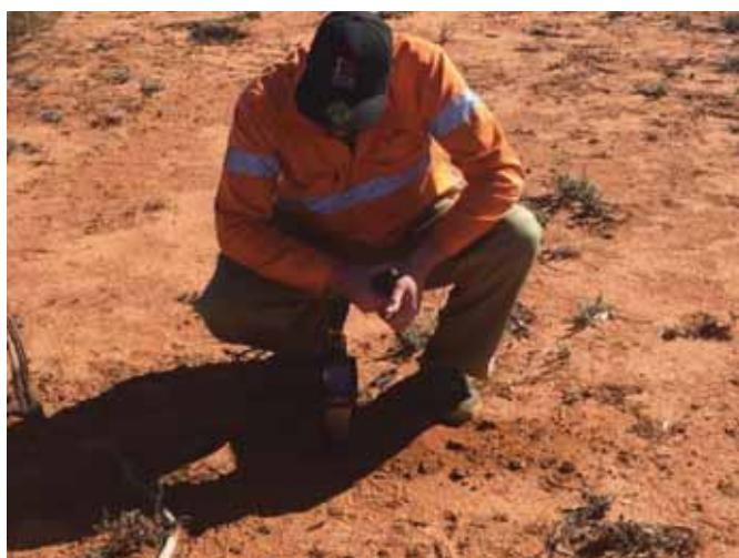
**Figure 5** Surficial geochemical sampling within the Canegrass project using the Delta instrument
